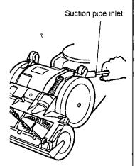
3) If the obstruction occurs in the suction pipe inlet, it can be removed with care as shown
